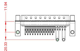
**OPERATING TEMPERATURE:** -55°C ~ 125°C **POWER/CO-AX CONTACT RATING:** (IF PRESENT) SIGNAL CONTACT CURRENT RATING: 5A PER CONTACT SIGNAL CONTACT RESISTANCE:  $10m\Omega$  MAX. **INSULATOR RESISTANCE:** 5000MΩ min.
