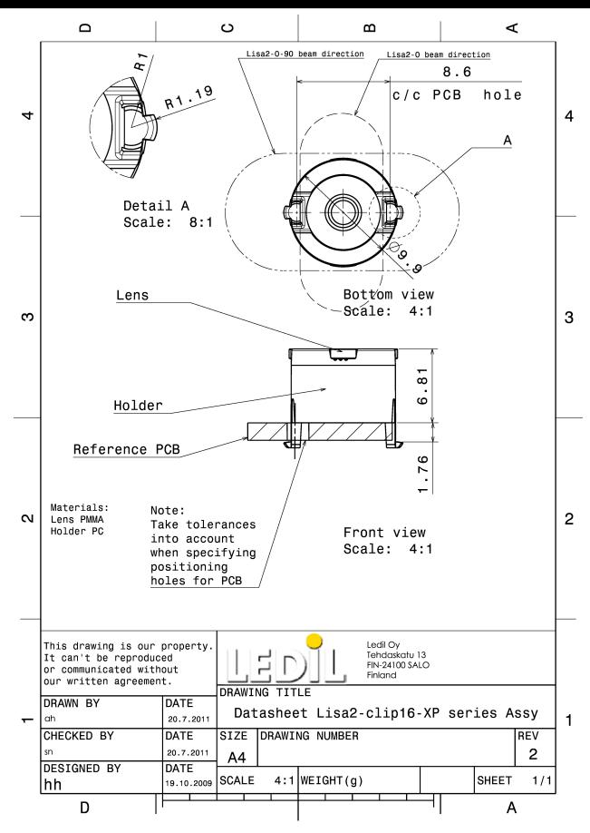
See also our general installation guide: <a href="www.ledil.com/installation\_guide">www.ledil.com/installation\_guide</a>
