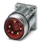
Device connector for front wall, straight, shielded: yes, for standard and SPEEDCON interlock, M40, No. of pos.: 4+4+4+PE / 3+N+PE, type of contact: Pin, Crimp connection, Axial O-ring, 4x Ø4,2, flange dimensions: 40 mm x 40 mm
