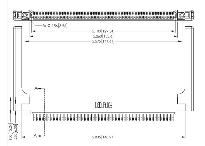
160 [4.06] POINT OF CONTACT 330[8.38] CARD SLOT **SECTION A-A**
