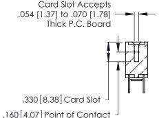
INSULATOR MATERIAL: THERMOPLASTIC POLYESTER, UL 94V-0 CONTACT MATERIAL; COPPER, NICKEL, TIN ALLOY CA-725
