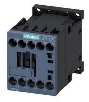
Power contactor, AC-3 16 A, 7.5 kW / 400 V 1 NO, 277 V AC, 60 Hz 3-pole, Size S00 screw terminals
