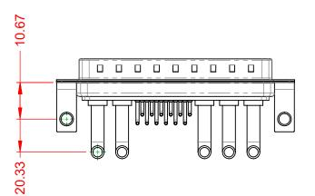
OPERATING TEMPERATURE: $-55^{\circ}C \sim 125^{\circ}C$ POWER/CO-AX CONTACT RATING:40A (CURRENT)(IF PRESENT)SIGNAL CONTACT CURRENT RATING:5A PER CONTACTSIGNAL CONTACT RESISTANCE: $10m\Omega$  MAX.INSULATOR RESISTANCE: $5000M\Omega$  min.DIELECTRICDIELECTRIC
