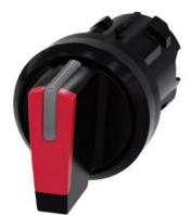
Selector switch, illuminable, 22 mm, round, plastic, red, selector switch, short, 3 switch positions I>O<II, momentary contact type, actuating angle 2x45°, 10:30h/12h/13:30h, with laser labeling, upper case and lower case, always upper case at beginning of line
