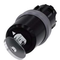
key-operated switch Siemens, 22 mm, round, plastic with metal front ring, lock number SSG10, with 2 keys, 2 switch positions O-I, latching, actuating angle 90°, 10:30h/13:30h, key removal O, with laser labeling, inscription or symbol customer-specific selection with SIRIUS ACT configurator (CIN)
