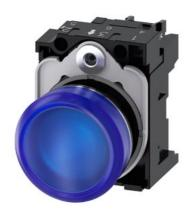
Indicator lights, 22 mm, round, metal, shiny, blue, lens, smooth, with holder, LED module with integrated LED 24 V AC/DC, screw terminal, with laser labeling, symbol number according to, ISO 7000 or IEC 60417
