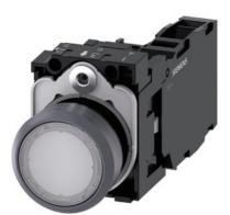
Illuminated pushbutton, 22 mm, round, plastic with metal front ring, white, pushbutton, flat, momentary contact type, with holder, 1 NO+1 NC, LED module with integrated LED 110 V AC, screw terminal, with laser labeling, lower case
