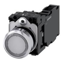
Illuminated pushbutton, 22 mm, round, Metal, shiny, clear, pushbutton, flat, momentary contact type, with holder, 1 NO+1 NC, LED module with integrated LED 230 V AC, screw terminal, with laser labeling, upper case and lower case, always upper case at the beginning of the word
