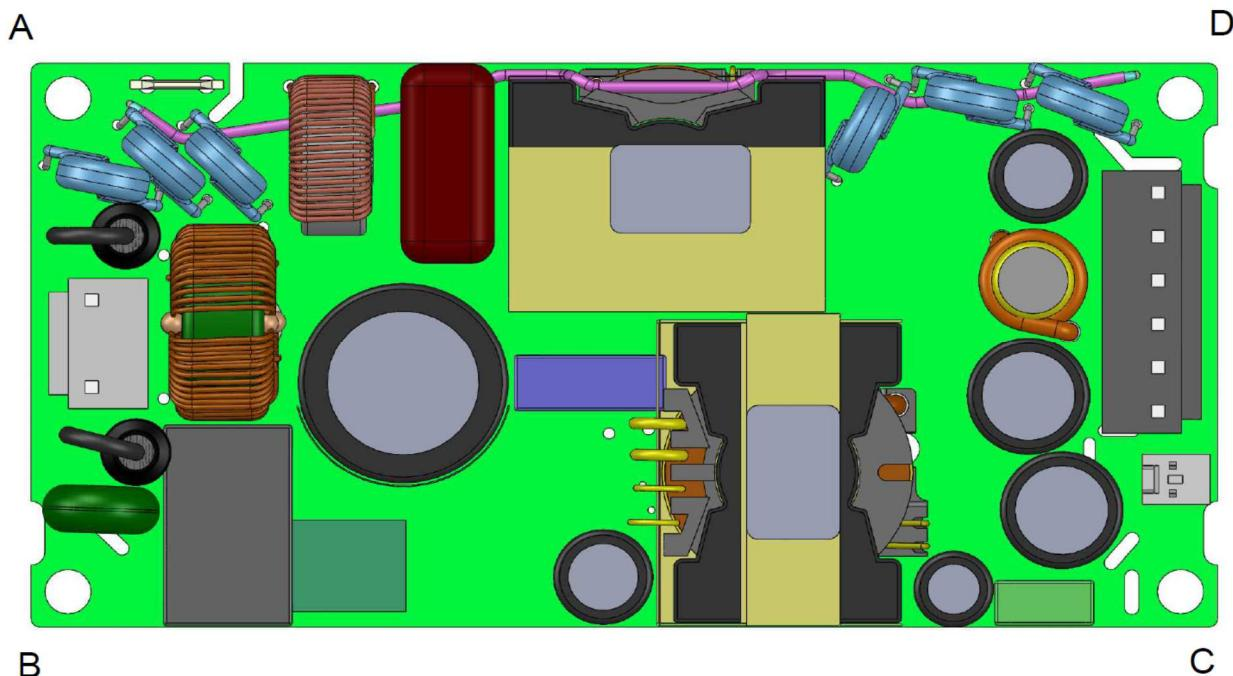
All four mounting points (A, B, C, D) should be used to support the unit.
