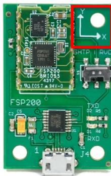
Figure 10: FSP200 Serial/USB Adapter Board Orientation
