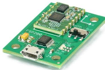
Figure 1: FSP200 USB Serial adapter board
