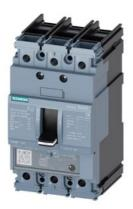
circuit breaker 3VA5 UL frame 125 breaking capacity class S 25kA @ 480 V 3-pole, line protection TM230, FTAM, ln=110A overload protection lr=110A fixed short-circuit protection li=5...10 x ln cable connection on both sides
