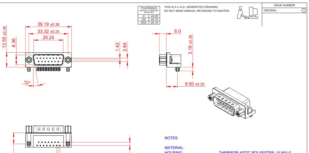
HOUSING: SHELL: CONTACT: THERMOPLASTIC POLYESTER, UL94V-0 STEEL, NICKEL PLATED COPPER ALLOY, 30µ GOLD PLATING
