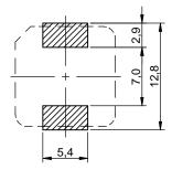
no sensitive traces underneath the component
