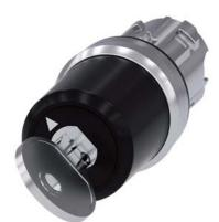
Key-operated switch BKS, 22 mm, round, metal, shiny, lock number S1, with 2 keys, 2 switch positions O-I, latching, actuating angle 90°, 10:30h/13:30h, key removal I, with laser labeling, upper case and lower case, always upper case at beginning of line
