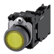
Illuminated pushbutton, 22 mm, round, plastic with metal front ring, yellow, pushbutton, flat, momentary contact type, with holder, 1 NO+1 NC, LED module with integrated LED 24 V AC/DC, spring-type terminal, with laser labeling, upper case and lower case, Always upper case at the beginning of the word
