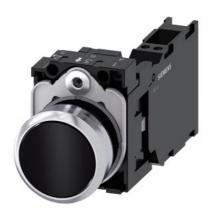
Pushbutton, 22 mm, round, metal, shiny, black, pushbutton, flat, momentary contact type, with holder, 1 NO+1 NC, spring-type terminal, with laser labeling, inscription or symbol Customer-specific selection with SIRIUS ACT configurator (CIN)
