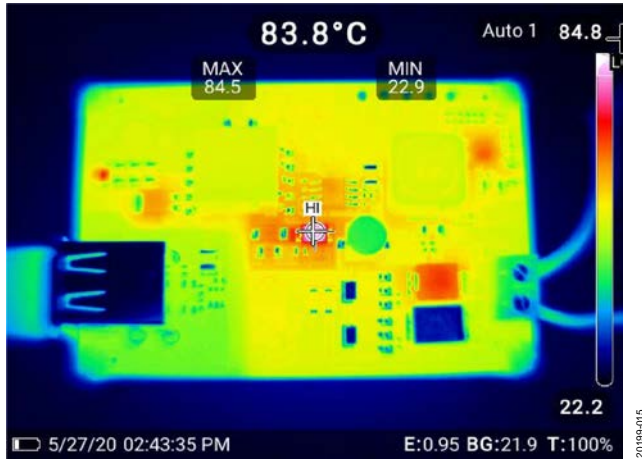
Figure 15. Thermal Image of EVAL-CN0509-EBZ at 5.62 V, 2 A Output Charging a Load for One Hour
