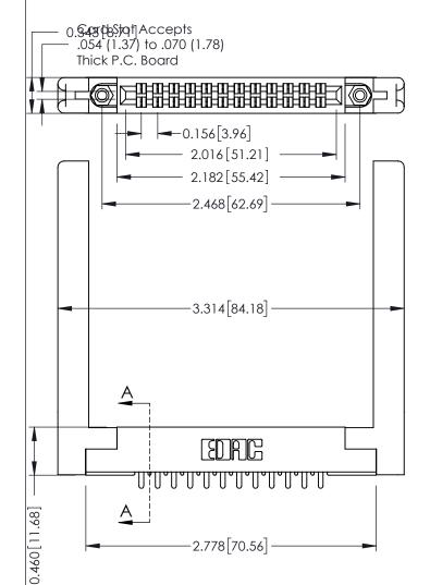
0.090[2.29] Point of Contact 305 ENG MASTER 305 / 315 / 355 Card Edge Connector J.LEE DATE: SEPT. 21/09 Part Number: 315-024-521-258 SHEET 1 OF 2 NTS
