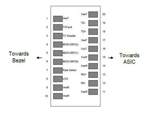
Pin-out of connector Block on Host board
