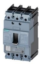
circuit breaker 3VA5 UL frame 125 breaking capacity class H 65kA @ 480 V 3-pole, line protection TM230, FTAM, In=25A overload protection Ir=25A fixed short-circuit protection Ii=6...12 x In cable connection on both sides
