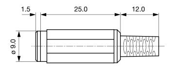
Cable diameter max. 4.0 mm
