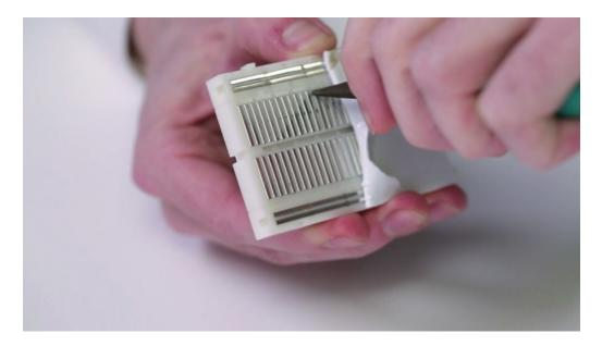
Beneath all those holes, a breadboard houses an army of springy metal clips which hold component leads in place while providing electrical connections between them.
