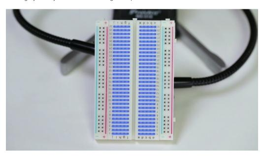
When we place a component on a breadboard, we're essentially wiring it into one of those internally connected rows.
