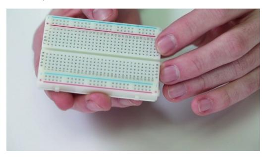
And in reality, a circuit usually exists on some type of circuit board - like say, a breadboard for example.
