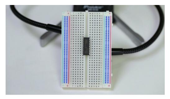
The two columns of holes along the sides are connected vertically.
