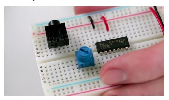
You can find a lot of components that are "breadboard friendly", meaning that their lead-spacing matches up nicely with a breadboard, so they pop right into place.
