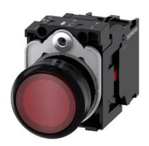
Illuminated pushbutton, 22 mm, round, plastic, red, pushbutton, flat, momentary contact type, with holder, 1NC, LED module with integrated LED 230 V AC, screw terminal, with laser labeling, lower case
