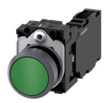
Pushbutton, 22 mm, round, plastic with metal front ring, green, pushbutton, flat, momentary contact type, with holder, 1 NO+1 NC, screw terminal, with laser labeling, upper case and lower case, always upper case at beginning of line
