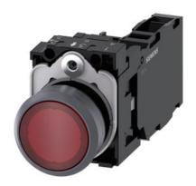
Illuminated pushbutton, 22 mm, round, plastic with metal front ring, red, pushbutton, flat, momentary contact type, with holder, 1 NO+1 NC, LED module with integrated LED 24 V AC/DC, screw terminal, Z=20-unit packaging
