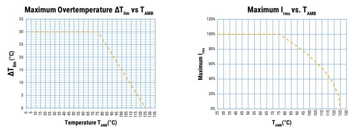
$T_{AMB}$  is the maximum ambient temperature surrounding the capacitor or hottest contact point (e.g. tracks), whichever is higher, in the worst operation conditions in °C.
