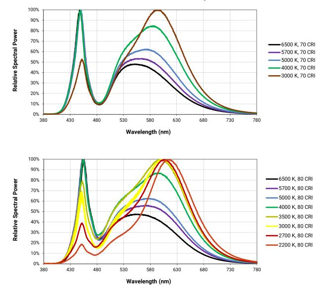
The following graphs are the result of a series of pulsed measurements at 800 mA and T<sub>1</sub> = 85 °C.
