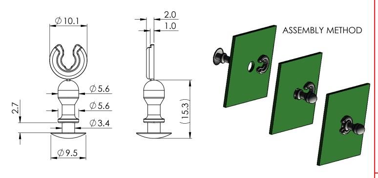
TO FIT A Ø5.8 - 6.4 HOLE IN A 1.6 THICK PANEL
