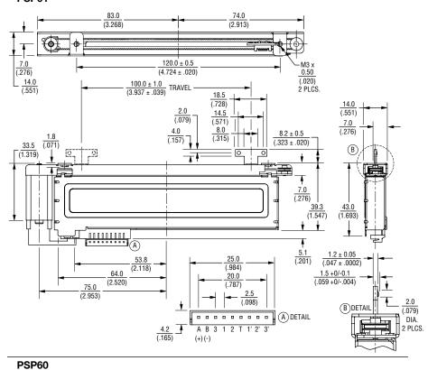
PSP Series Motorized Master Slide Potentiometer
