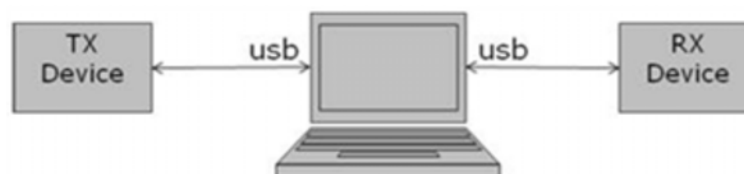
Figure 5. Connection setup 2: 2 PCs with S2-LP-DK GUI
