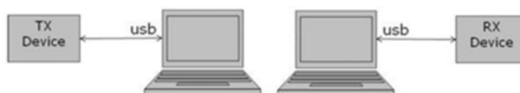
Figure 5. Connection setup 2: 2 PCs with S2-LP-DK GUI
