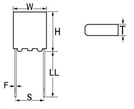
**General Information** Series T340 Dielectric MnO2 Tantalum Style Radial Molded Radial, Solid Tantalum, Molded Description RoHS Yes Termination Tin AEC-Q200 No Construction Molded Includes Standoff Height of 0.38 +/- 0.13mm. Miscellaneous Longest Lead Is Positive. Notes
