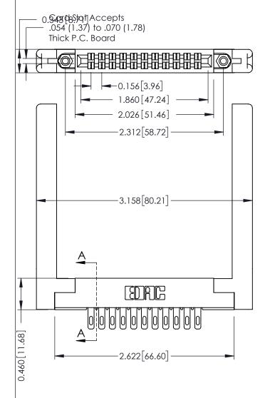
0.295[7.49] Card Slot ECTION 0.090 [2.29] Point of Contact 305 ENG MASTER 305 / 315 / 355 Card Edge Connector J.LEE DATE: SEPT. 21/09 Part Number: 315-022-500-258
