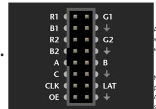
A **32x16** panel uses this pin arrangement. The labels might be slightly different, or the pins might not be labeled at all...but in either case, use this image for reference.
