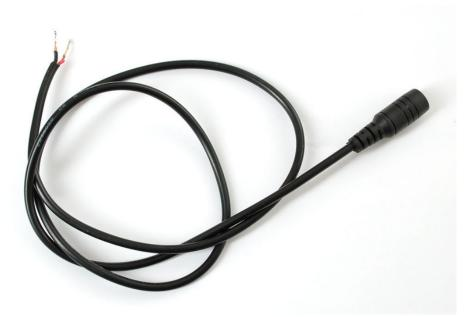
Solder both pins correctly to the power port. Make sure you get this right because there is no protection diode!
