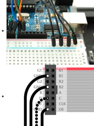
**32x32** and **64x32** matrices require **three** ground connections. **32x16** matrices have **four**.
