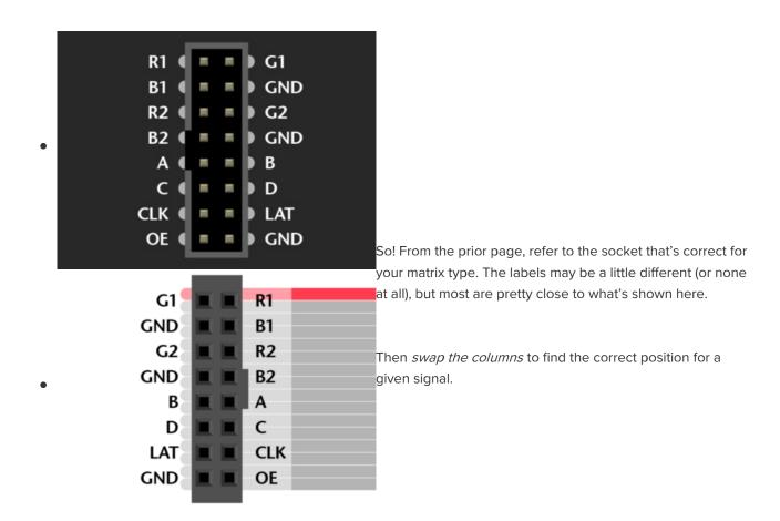
**Either end of the ribbon cable can be plugged into the matrix INPUT socket.** Notice below, the "key" faces the same way regardless.
