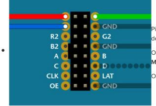
Pins **R1**, **G1** and **B1** (labeled R0, B0 and G0 on some matrices) deliver data to the **top half** of the display.
