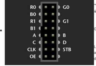
"Variant B" for 32x32 and 64x32 panels. The wiring is identical to Variant A above, only the labels are different.
