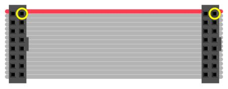
Either end of the ribbon cable can be plugged into the matrix INPUT socket.
