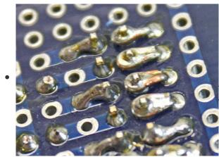
Depending on the make and model of proto shield, some pins are designed to connect in short rows. Others don't. For the latter, strip a little extra insulation and bend the wire to wrap around the leg of the socket from behind, then solder.
