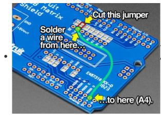
The shield requires a small modification to work with the Adafruit **Metro M4**:
