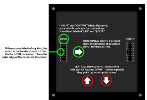
The arrangement of pins on the INPUT connector varies with matrix size and the batch in which it was produced...
