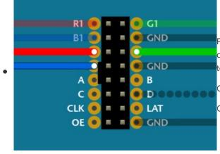
Pins **R2**, **G2** and **B2** (labeled R1, G1 and B1 on some matrices) deliver data to the **bottom half** of the display. These connect to the next three Arduino pins...
