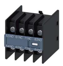
Auxiliary switch on the front, 2 NO + 2 NC Current path 1 NO, 1 NC, 1 NC, 1 NO for contactor relays Size S00 Ring cable lug connection 53/54, 63/64, 73/74, 83/84 Physically coded; only with contactor relays 3RH2140\* and 3RH2440\* can be combined (according to EN 50011)
