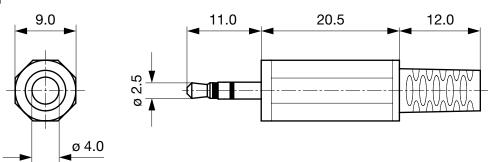
Cable diameter max. 4.0 mm
