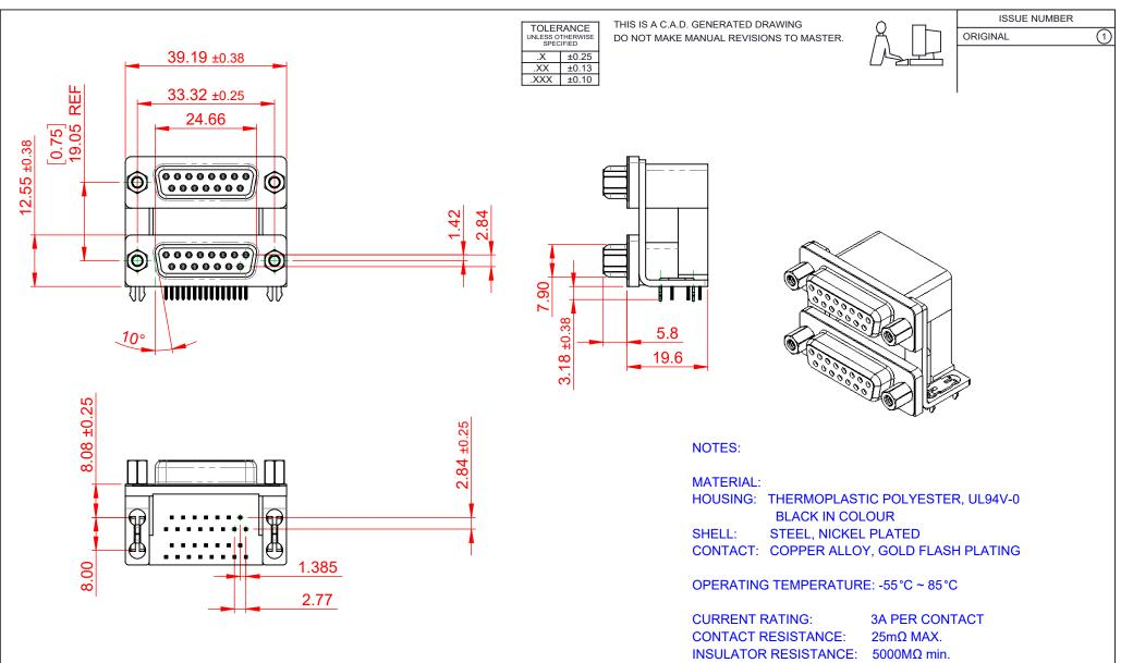
DIELECTRIC WITHSTANDING VOLTAGE: 1000V AC rms
