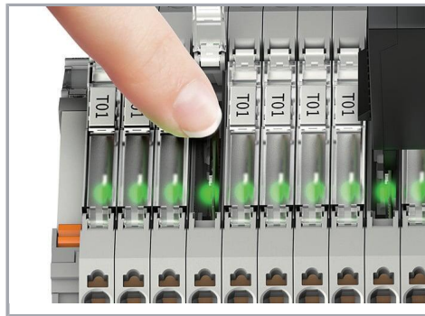
Configuration via push/slide switch
