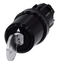
key-operated switch Siemens, 22 mm, round, plastic, special lock, with 2 keys, 3 switch positions I>O<II, momentary contact on the left, latching on the right, actuating angle  $2x45^\circ$ , 10:30h/12h/13:30h, key removal O
