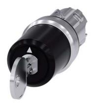
key-operated switch Siemens, 22 mm, round, metal, shiny, lock number SSG10, with 2 keys, 3 switch positions I>O<II, momentary contact on the left, latching on the right, actuating angle 2x45°, 10:30h/12h/13:30h, key removal O, Z=50-unit packaging
