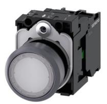
Illuminated pushbutton, 22 mm, round, plastic with metal front ring, white, pushbutton, flat, momentary contact type, with holder, 1NO, LED module with integrated LED 110 V AC, screw terminal, with laser labeling, lower case
