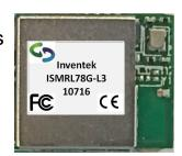
The module provides UART, I<sup>2</sup>C, and CSI interfaces enabling easy connection to an embedded design. The low-cost, the small foot-print design (11mm x 13 mm) and the ease of design-in make it ideal for a wide range of embedded BLE applications.
