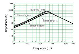
AC Line Filters – Common Mode SSR Coils, 21HS Series, Wide Range Impedance Series
