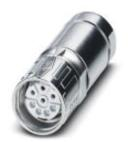
Cable connector, SPEEDCON locking, M23, number of positions: 5+PE, type of contact: Socket, Crimp connection, shielded: yes, cable diameter range: 9 mm ... 12 mm
