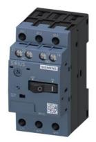
Circuit breaker size S00 for motor protection, CLASS 10 A-release 0.45...0.63 A N-release 8.2 A Screw terminal Standard switching capacity with transverse auxiliary switch 1 NO+1 NC
