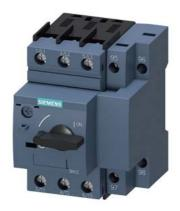
Circuit breaker size S0 for motor protection, CLASS 10 with overload relay function A-release 27...32 A N-release 400 A screw terminal Standard switching capacity
