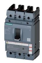
circuit breaker 3VA5 UL frame 250 breaking capacity class M 35kA @ 480 V 3-pole, line protection TM230, FTAM, In=125A overload protection Ir=125A fixed short-circuit protection Ii=5...10 x In UL 489 SB (naval), 50° C without connection
